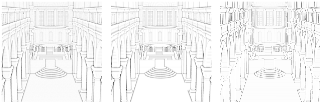
Figure 6.1: Demonstration of the similarities between Screen Space Ambient Occlusion and Volumetric Obscurance. The left image uses 33 point samples and runs at 156 fps. The middle image uses nine line samples and runs at 210 fps. The rightmost image uses a single line sample and runs at 240 fps.
