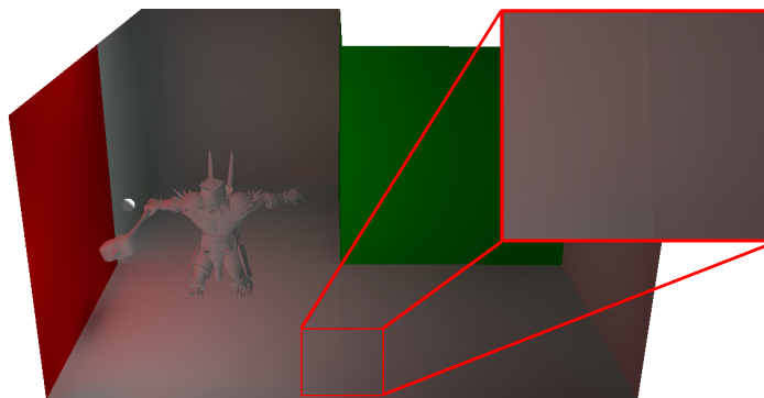
Figure 4.12: Indirect lighting on our example map without light map padding. When we do not use light map padding, we end up with discontinuities between our blocks.
